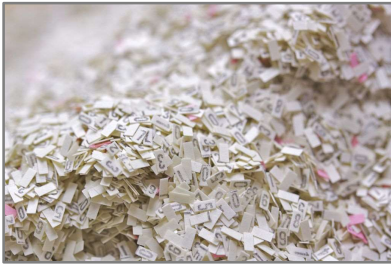
Chads from punched cards. Each chad is about 1/8 inch (3 mm) long. Marcin Wichary. CC BY 2.0
