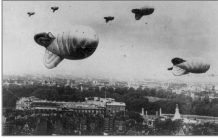
Barrage balloons over London during World War II. Barrage balloons held steel cables above the ground to endanger enemy aircraft. Their shape retained more stability in wind than spherical balloons.
